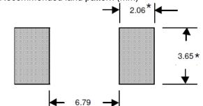
\* suggest to enlarge for wave soldering.
